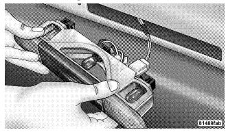
3. Remove connector from housing tab for more clearance.
